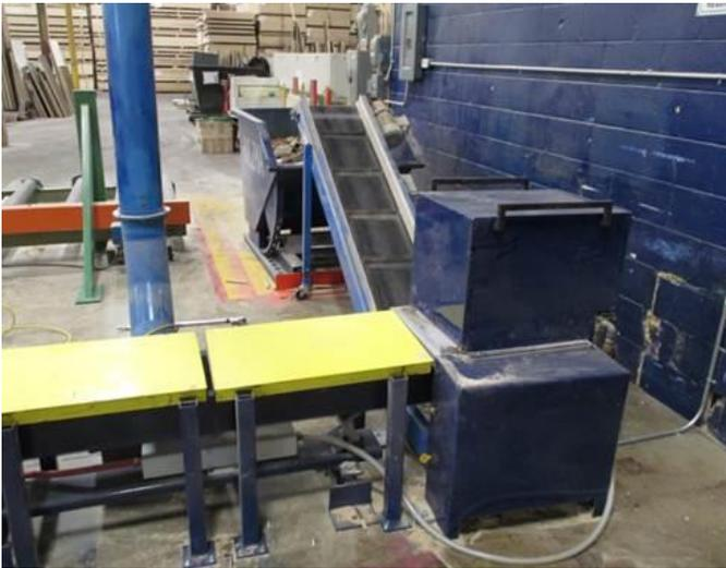
**HOLZMA grinder replacement:** The grinder's 30 hp motor was running 18 hours per day but used only 35 percent of the time. This new pneumatic guillotine replaced the grinder and operates only when needed. Estimated annual savings: 41,355 kWh or \$6,616.
