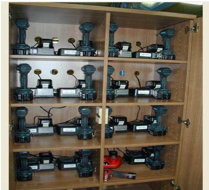
**Air drill replacement: Charging station for the cordless tools that replaced the air drills. Estimated annual savings: 36, 832 kWh or \$5,893.**
